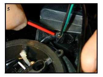
Pull some of the factory wire harness into the mirror housing. Using the shorter of the two wires from the kit for the driver side door, guide the end without the connector into the sheath alongside the existing wire.
